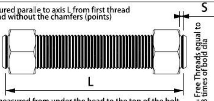
Hex bolts are measured from under the head to the top of the bolt
